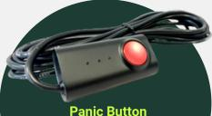
For the machine operator to manually send recordings for review to VUEhub i.e. a situation happening that may not have triggered the cameras.
