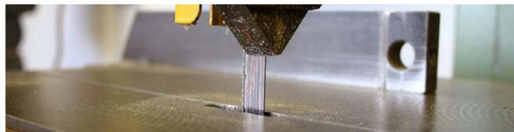
A band saw is a common item of machinery found in woodworking premises. It uses a blade consisting of a continuous band of toothed metal rotating on opposing wheels to cut material which in this case will be timber. Fixed dust extraction can be installed to reduce the build-up of wood waste and sawdust.
