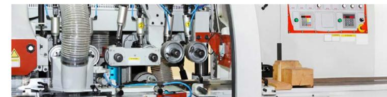
Designed to shape wood into profiles. It's typically used for creating grooves, rebates and bevels. Various tooling is used on the spindle to create the necessary cut.
