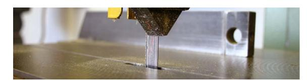
A band saw is a common item of machinery found in woodworking premises. It uses a blade consisting of a continuous band of toothed metal rotating on opposing wheels to cut material which in this case will be timber. Fixed dust extraction can be installed to reduce the build-up of wood waste and sawdust.
