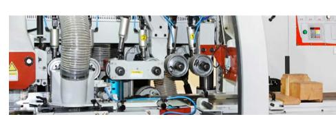
Designed to shape wood into profiles. It's typically used for creating grooves, rebates and bevels. Various tooling is used on the spindle to create the necessary cut.
