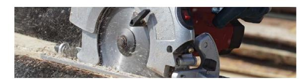
A rip saw is a special type of powered saw that cuts in the direction of the grain. The teeth on the saw are specially designed so that they effectively scrape away the wood rather than cutting it, acting like small chisels.
